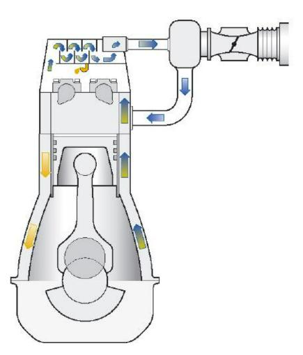
In the case of the three new NG6 engines, there are two methods employed. The N54 engine does not use a crankcase ventilation valve and oil is separated using the "cyclonic method".
