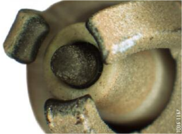
The spark plug above shows a normal wear pattern for a spark plug with high mileage. Spark plug is due for replacement.
