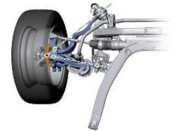
The pivot points of the control arm or wishbone and tension strut at the swivel bearing can therefore be selected such that no space problems are encountered for the brake system.
