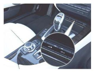
The green LED in the button lights up during the opening/closing operation. The red LED signals an operating error or incorrect conditions (e.g. luggage compartment partition not in lower position). The red LED flashes as soon as the retractable hardtop is in an intermediate position and not operated. The LED flashing does not indicate a fault. The flashing LED draws attention to the fact that the vehicle cannot be driven in this situation.
