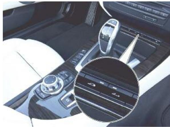
The green LED in the button lights up during the opening/closing operation. The red LED signals an operating error or incorrect conditions (e.g. luggage compartment partition not in lower position). The red LED flashes as soon as the retractable hardtop is in an intermediate position and not operated. The LED flashing does not indicate a fault. The flashing LED draws attention to the fact that the vehicle cannot be driven in this situation.
