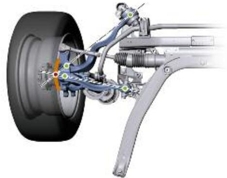
The pivot points of the control arm or wishbone and tension strut at the swivel bearing can therefore be selected such that no space problems are encountered for the brake system.
