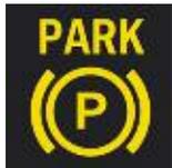
**E89 Indicator lamp, parking brake fault**
